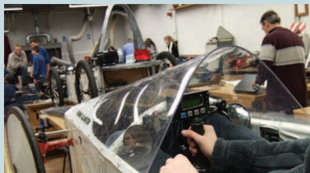
A lever is used to steer Rotary Racer
