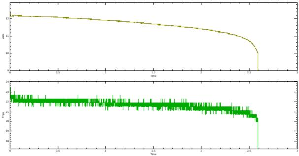
Illustration 2: Typical Yuasa battery discharge curve
