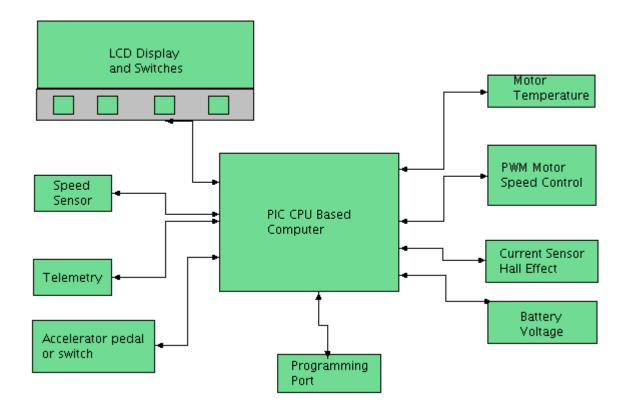
As an example of its use in the Rotary Racer, the computer can measure the following car parameters.
