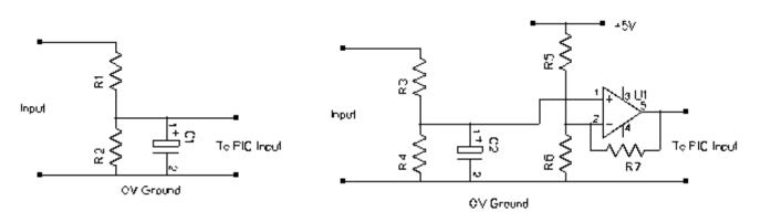
Two of the inputs, designed for the current and temperature inputs, have the same basic input circuit but have a following operational amplifier that can scale and offset the voltage as required. R5, R6 and R6 can be adjusted for voltage offset and gain. By default the operational amplifier is set for a gain of 1 and no offset.
