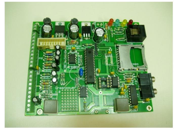
The board was designed after playing with a prototype system using PicAxe computer modules on the Rotary Racer Greenpower car. The circuit design was done by a parent, the PCB was laid out by a parent with the pupils laying out some of the tracks. The PCB was sent out to a PCB production house for manufacture. The components were soldered in place by the pupils with help by the parents. Test LED code was done by some of the pupils.
