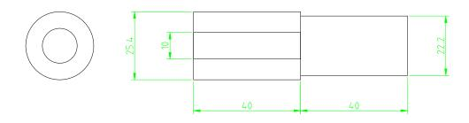
Rear Stub Axles Aluminium bar 25.4mm diameter Hole drilled 10.2mm threaded 12mm x 1.75mm Stub close fit into 25.4mm (1.6mm thickness) steel tube
