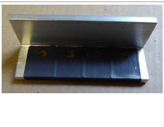
The white/beige pads are fine, but the black pads are not fully electrically insulating and can, if the screws are tightened hard (as they should be) cause the MOSFET's/heat-sink to heat up as current will flow through them. Also any burs at all are likely to cause shorts from the MOSFET to the heat-sink.
