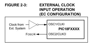
The ECIO Oscillator mode functions like the EC mode, except that the OSC2 pin becomes an additional general purpose I/O pin. The I/O pin becomes bit 6 of PORTA (RA6). Figure 2-4 shows the pin connections for the ECIO Oscillator mode.
