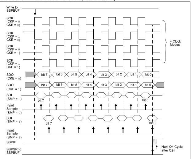
FIGURE 17-3: SPI MODE WAVEFORM (MASTER MODE)
